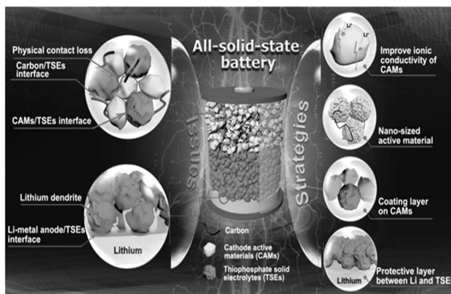
FIGURE 6.2 Summary of the interfacial issues in ASSBs with TSEs and the corresponding strategies. Reproduced from Ref. Wang et al. (2020) with permission. Copyright 2020 Elsevier.
