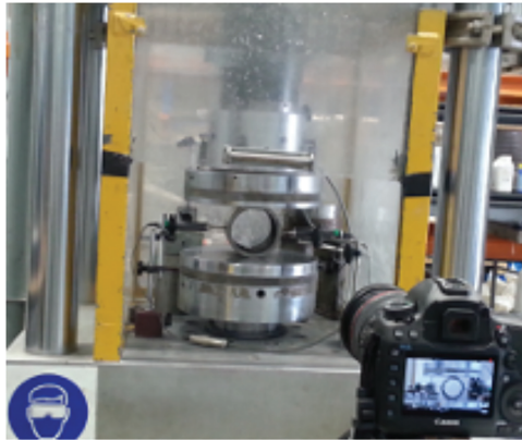
Figure 4.12 Set-up of crush ring test.
