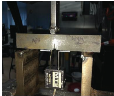
Figure 3.19 Test set-up for fracture toughness.
