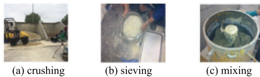
Figure 4.1 Preparation of test soil (a) crushing, (b) sieving and (c) mixing.
