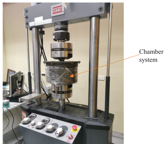
Figure 6.4 Set-up of combined corrosion and fatigue test.
