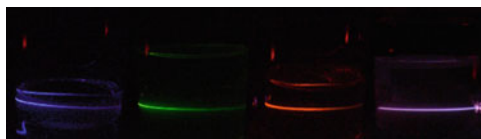
Fig. 3 Photographic picture of upconverting nanocrystals with four different colours (no filters or overexposure were used). Excitation: 980 nm laser diode. Reprinted with permission from [26]. Copyright 2008 American Chemical Society
