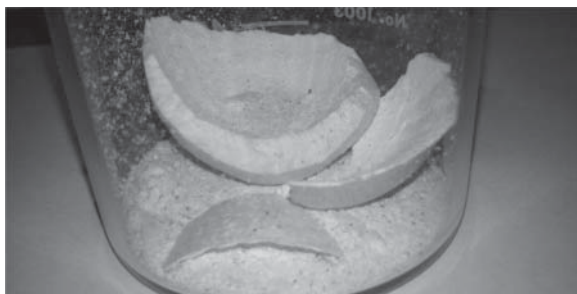
Figure 19.7 Image of a poly(HEMA- co -EGDMA) polymer network synthesized in \text{scCO}_2 . Two distinguishable materials were obtained because of separation of the reaction mixture during the synthesis in two phases: (i) a hard and brittle polymer network of hemispherical shape, which corresponds to the shape of the bottom of the reactor vessel, and (ii) a soft fluffy powder polymer network polymerized in the upper section of the reactor.
