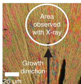
Figure 11.3 Spherulite observed under polarized optical microscopy. The approximate region probed by the X-ray is indicated by the circle. The center of the spherulite lies outside the photographed area. “Growth” indicates the radial growth direction. Source: Aou and Hsu [18].
