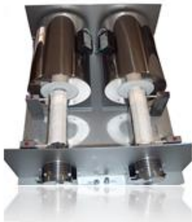
Figure 12: Eraly pyrolyser with multi tube (here two) to analyse two different samples (the main cover was taken off for the picture)
