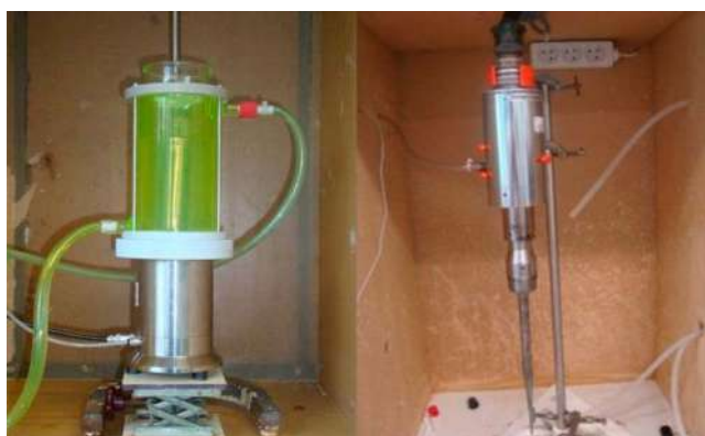
Figure 8.3 Cup horn system (left) and ultrasonic probe (right) in the lab.
