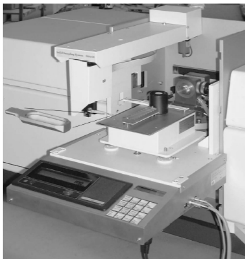
Figure 2. Solid sampling autosampler (with kind permission of Analytik Jena SSA 61)
