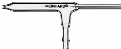
Figure 18. The high efficiency nebulizer (HEN). Courtesy of Meinhard Glass Products.
