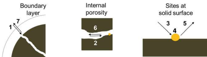
Fig. 3.7 Fundamental steps of a catalytic fluid–solid reaction performed in a porous catalyst. Adapted from Piumetti and Russo [3]
