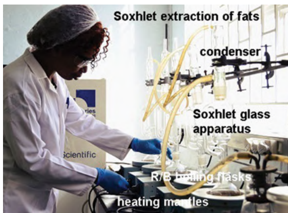
Fig. 1.2: Soxhlet fat extraction.
