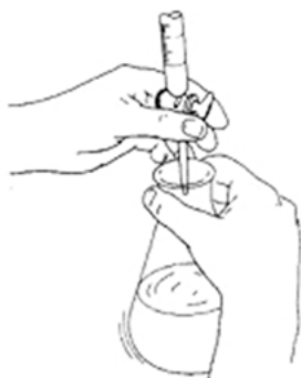
Fig. 21.3: How to read a burette.
