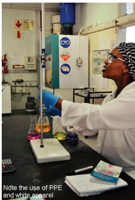
Fig. 21.2: Adjusting the height of burette for volumetric analysis.
