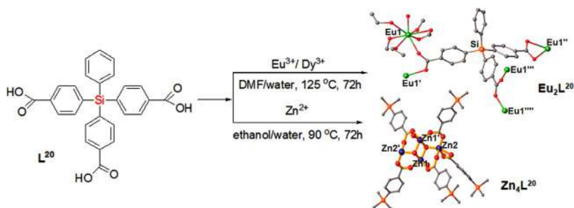
Fig. 20 Solvothermal procedures to obtain zinc(II) and lanthanide(III) MOFs.
