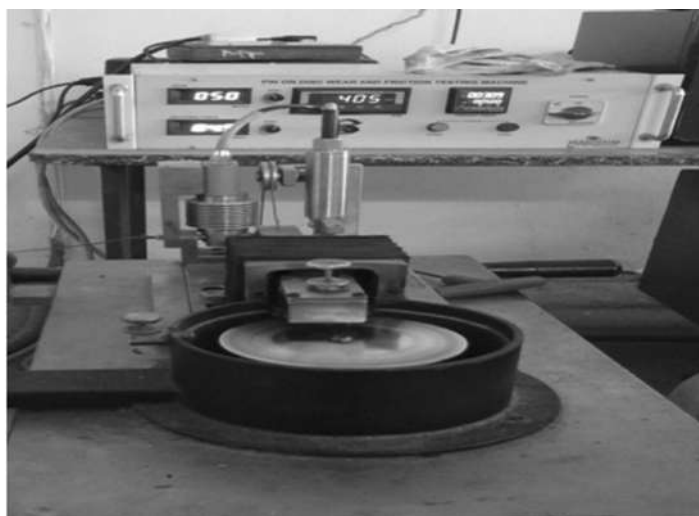
FIGURE 9.6 Pin-on-disc wear and friction testing.
