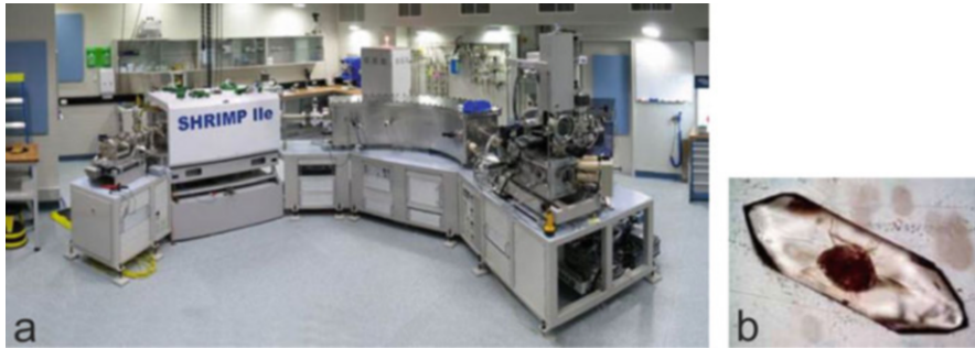
Fig. 4.1 Geochronometry. (a) SHRIMP device (© Geoscience Australia CC BY 4.0); (b) Ancient zircon crystal (© Geoscience Australia CC BY 4.0)
