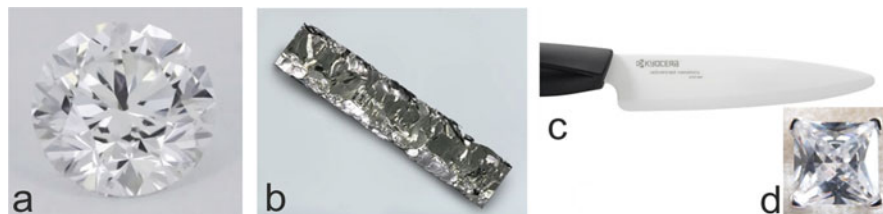
Fig. 1.1 The three materials. (a) Brilliant-cut zircon (With the kind permission of CARAT-Edelsteinhandel, Vienna); (b) Metallic zirconium (With the kind permission of Graz-Consulting, Prinzerdorf); (c) zirconium oxide ceramic knife (With the kind permission of Kyocera Feinceramics GmbH, Neuss); (d) Cut zirconia single crystal
