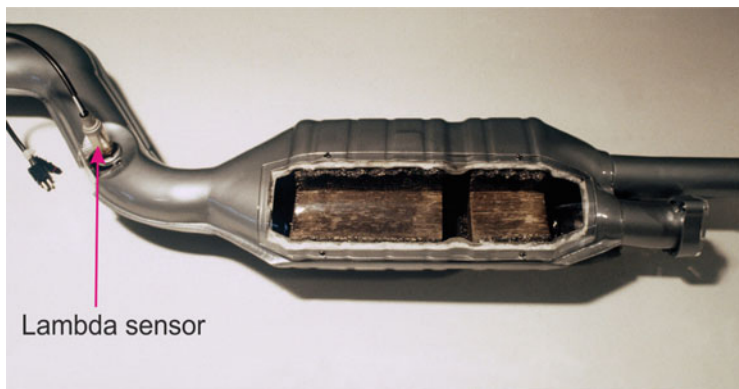
Fig. 19.1 Three-way catalytic converter with lambda sensor. (©Harry Melchert/dpa/picture alliance)
