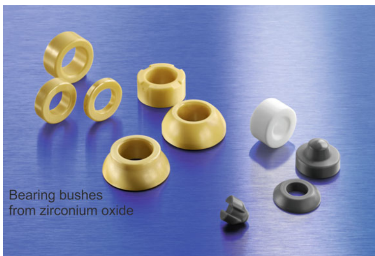
Fig. 17.2 Bearing bushes for exhaust gas flaps made of zirconium oxide ceramic. (With the kind permission of CeramTec GmbH, Plochingen)
