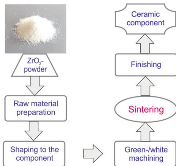
Fig. 12.1 Process steps of the sintering technique
