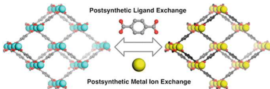
Fig. 9 Ligand and cation exchange for post-synthetic modifications in robust MOFs. Reprinted with permission from [67]. Copyright 2012 American Chemical Society
