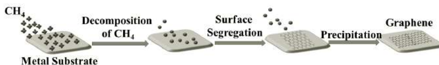
Figure 1.14. The illustration of the two-stage growth mechanism of graphene.
