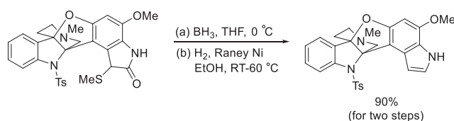
SCHEME 38 Hydrogenolysis of the methylthioxy group as a step in the total synthesis of (±)-phalarine.
