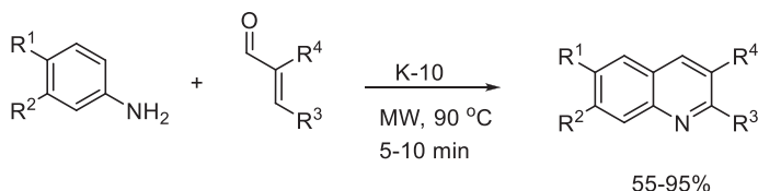
SCHEME 17 Microwave-assisted K-10 montmorillonite-catalyzed condensation-cyclialkylation of anilines with cinnamaldehydes.
