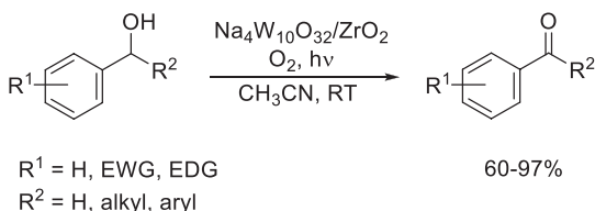
SCHEME 49 Zirconia-supported sodium decatungstate-catalyzed light activated oxidation of benzylic alcohols.
