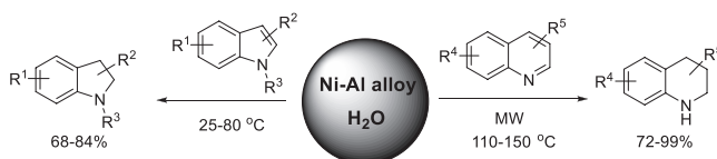
SCHEME 7 Hydrogenation of indoles and quinolines with Ni-Al alloy in water.
