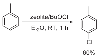
SCHEME 40 Zeolite-catalyzed chlorination of toluene.
