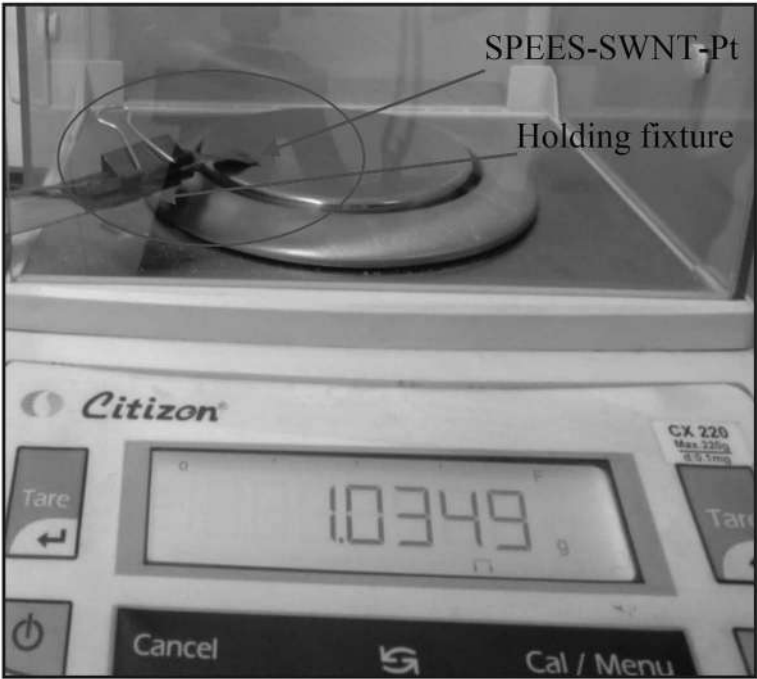
FIGURE 4.16 Testing setup for load characterization.
