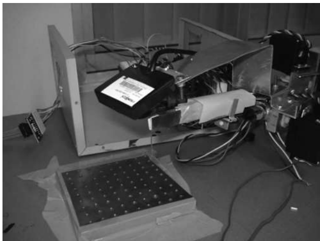
FIGURE 4.19 IPMC-based microgripper for handling objects [106].
