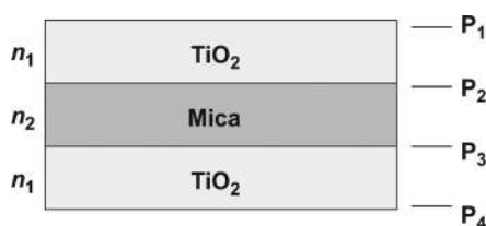
Figure 61.4: Schematic structure of a titanium dioxide mica pigment with the four existing interfaces ( P_1 – P_4 ).
