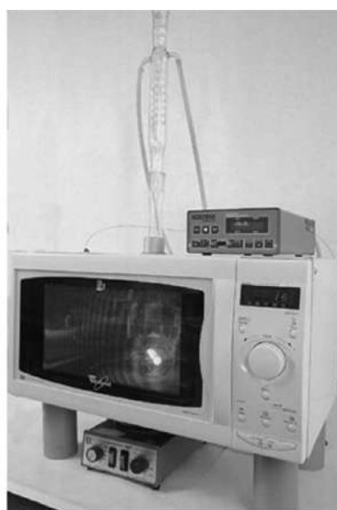
FIG. 18 (a) Photograph of the experimental setup. (b) A modified microwave oven for photochemistry. (Reproduced with permission from P. Klán, M. Hájek, V. Církva, The electrodeless discharge lamp: a prospective tool for photochemistry: Part 3. The microwave photochemistry reactor. J. Photochem. Photobiol. A 140 (3) (2001) 185–189.)
