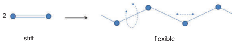
Figure i Illustration of configurational entropy gain during chain-growth polymerization.
