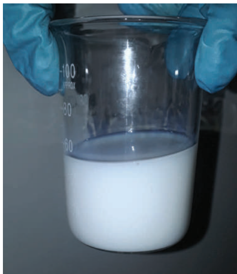
Figure 1.1 Polymer dispersion of poly(vinyl acetate-co-butyl acrylate) prepared by semi-batch seeded emulsion polymerization.
