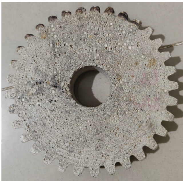
FIGURE 8.8 Fabricated \text{ZrO}_2 /PA6 composite gear.
