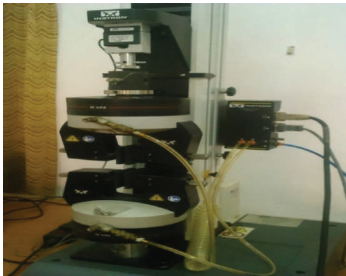
FIGURE 9.5 Universal testing machine with test specimen.
