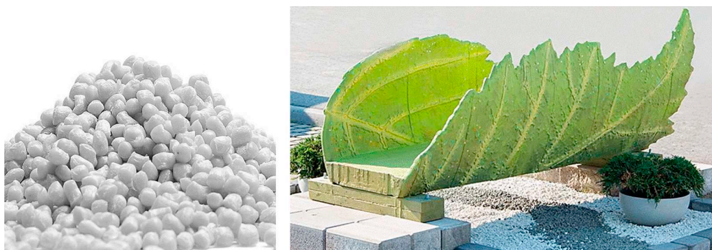
FIGURE 7.3 Left: granules of Formi 3D, cellulose/PLA composite for additive manufacturing. Right: leaf Bridge printed with filament made by Octofiber with UPM Formi 3D.
