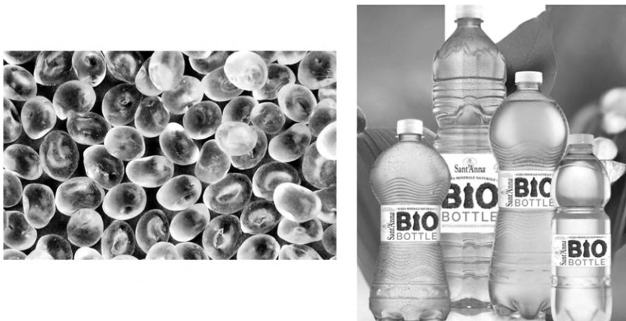
FIGURE 3.2 Left: pellets of Ingeo™ PLA. Right: water bottles made of PLA.
