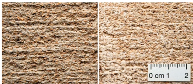
FIGURE 6.5 Cross section of spruce chips (SC) filled samples. Left: SC/cement/water. Right: SC/gypsum/water.
