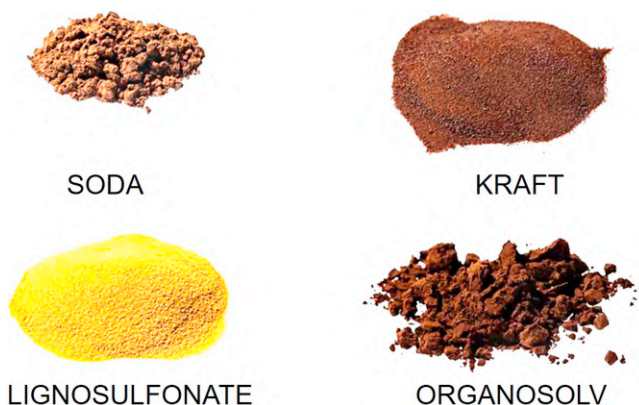
FIGURE 9.2 Pictures of typical technical lignins and their relative extraction process.
