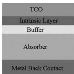
FIGURE 14.3 Physical structure of chalcogenide solar cells.
