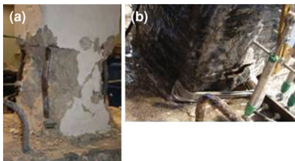
Fig. 5.6 a Disintegration of concrete and bar buckling. b Limited rupture of FRP jacket deformation capacity by approximately 10%
