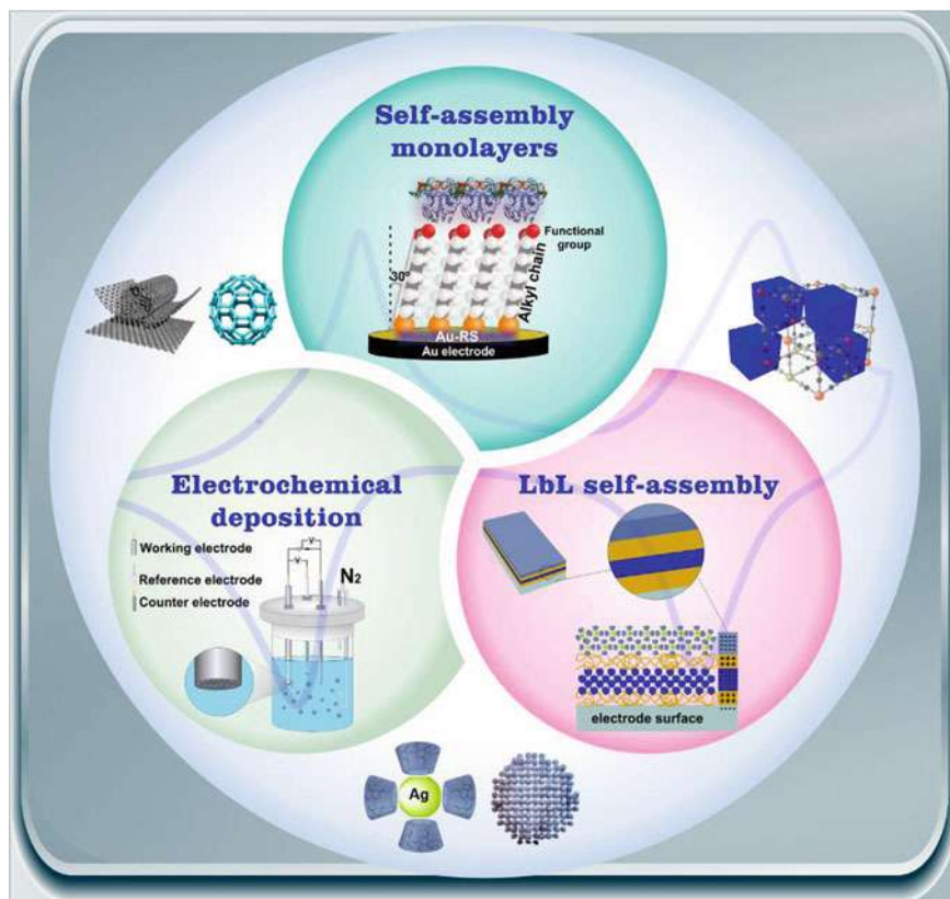
Fig. 3 Schematic representation of the main methods used to supramolecular assembly of building blocks onto electrode surfaces
