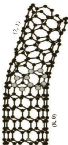
Figure 3.13 Atomic structure of an (8, 0)/(7, 1) intramolecular carbon nanotube junction. The large light-gray balls denote the atoms forming the heptagon–pentagon pair (Reprinted with permission from L. Chico et al., 1996 Pure carbon nanoscale devices: nanotube heterojunctions, 76, 971, copyright @ American Physical Society).
