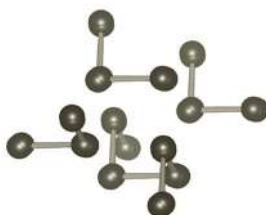
Figure 1.3 \text{Te}_8 trigonal crystallographic structure.
