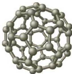
Figure 3.5 Buckminsterfullerene ( C_{60} ), zero-dimensional allotrope of carbon that are made from a graphene lattice in a spherical shape by the replacement of some hexagons with pentagons.
