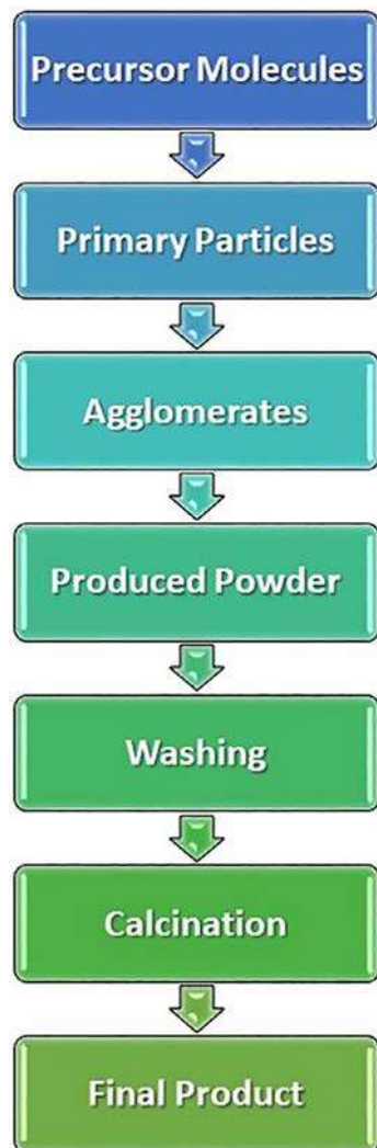
FIG. 8 Flame synthesis. Flowchart of the flame synthesis method.
