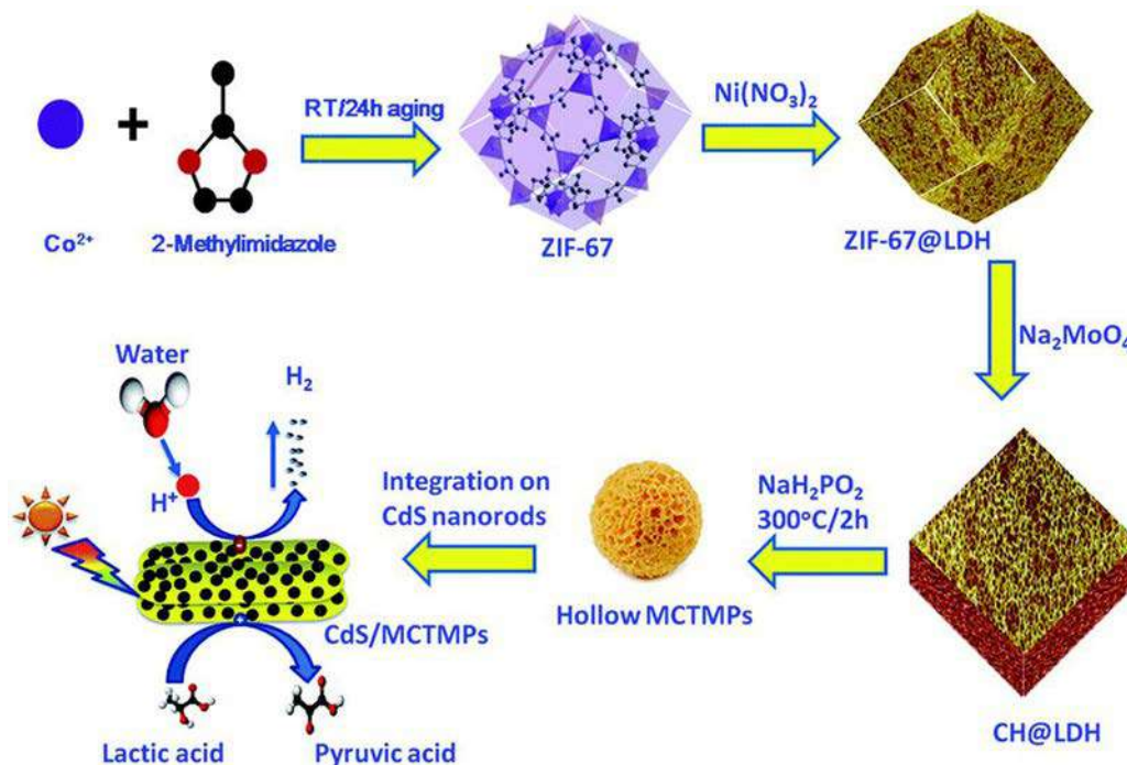
FIG. 8 Representative example of metal-organic framework template-engaged strategy. Schematic illustration of synthesis of multicomponent transition metal phosphide-CdS nanorod. From Amaranatha Reddy D, Kim HK, Kim Y, Lee S, Choi J, Jahurul Islam M. Multicomponent transition metal phosphides derived from layered double hydroxide double-shelled nanocages as an efficient non-precious co-catalyst for hydrogen production. J Mater Chem A 2016;4:13890–98. https://doi.org/10.1039/C6TA05741A .
