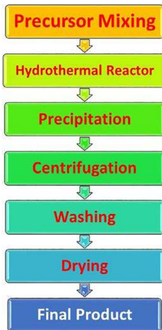
FIG. 4 Hydrothermal/solvothermal method. Elementary steps of the hydrothermal process for the preparation visible-photocatalyst.
