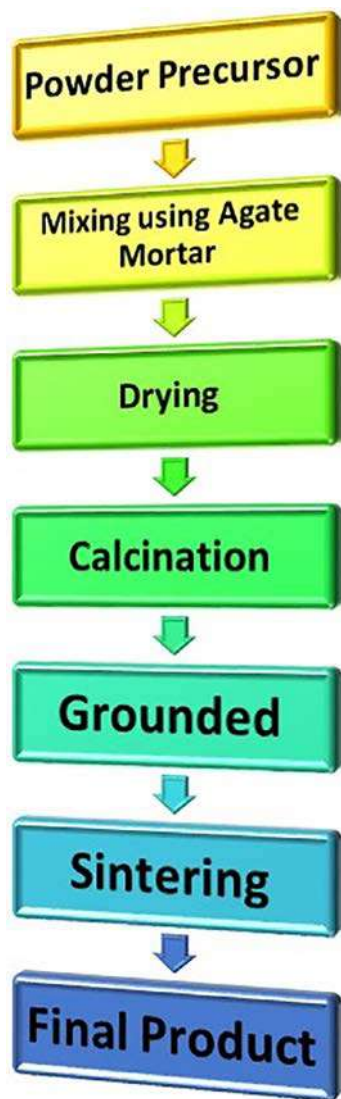
FIG. 5 Solid-state reaction method. Stepwise preparation of solid-state reactions method.
