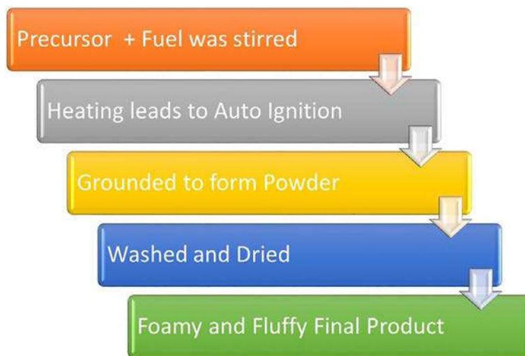
FIG. 6 Combustion reaction method. Flowchart for the combustion process for the preparation of visible light photocatalysts.
