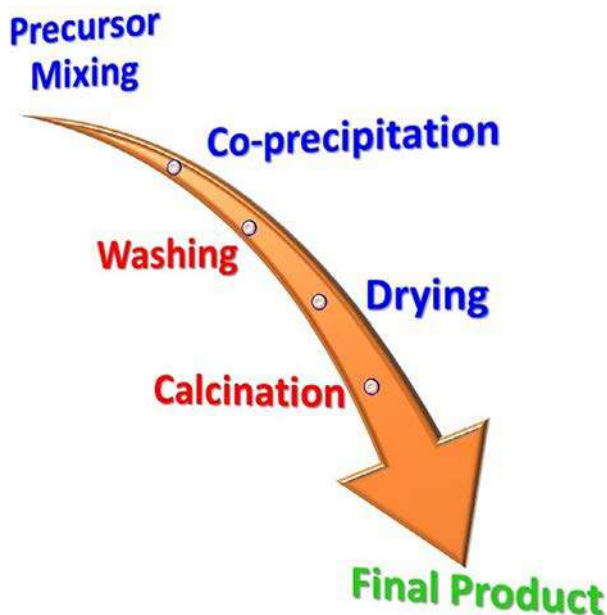
FIG. 2 Coprecipitation method. Flowchart of the coprecipitation process.
