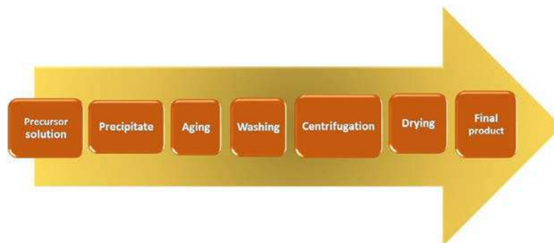
FIG. 1 Precipitation method. Flowchart of the precipitation process.
