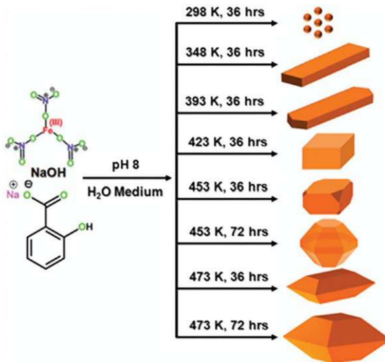
FIG. 11 Schematic presentation for the hydrothermal synthesis of various shapes \text{Fe}_2\text{O}_3 nanocrystals. From K. PA, K. KS, Asim B, Dukjoon K. Morphology evolution of single-crystalline hematite nanocrystals: magnetically recoverable nanocatalysts for enhanced facet-driven photoredox activity. Nanoscale 2016;8:365–77. https://doi.org/10.1039/C5NR06509G .
