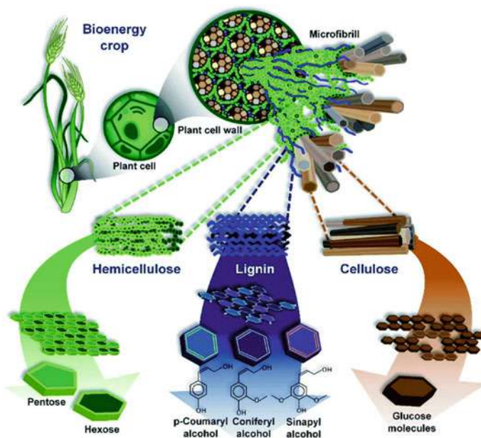
Fig. 3 The structure of the main components of lignocellulosic biomass. Adapted with permission from [18]
