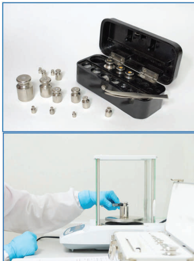
Figure 2.3 (a) A set of traceable weights. (b) Handling and using standard weights to check calibration and traceability. (Images used with permission of Shutterstock.com.)
