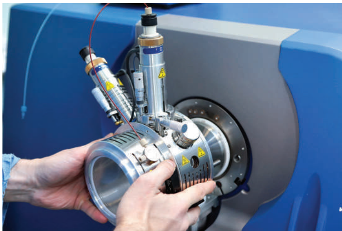
Figure 4.24 A commercial ambient ion source for LC. The circular metal piece just visible behind the source is the sample or skimmer cone. (Image used with permission of Shutterstock.com.)
