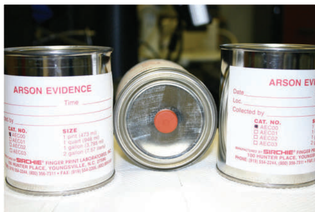
Figure 11.2 Evidence collection cans for fire debris analysis. The red circle in the center is a polymer septum that allows access to the contents without compromising the air-tight seal.
