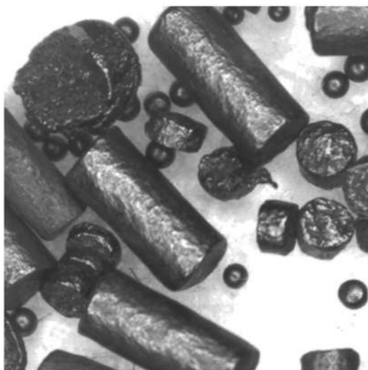
Figure 13.8 Shapes of propellant granules. Cylinders, disks, balls, and flakes are common in small arms propellants.
