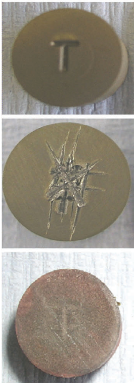
Figure 13.38 Restoration of an obliterated stamped letter using Fry's reagent. This is an example of over-stamping. (Reproduced with permission from Wightman, G. and J. Matthew, Restoration of stamp marks on steel components, Forensic Science International 180 (1) (2008) 32–36. Copyright Elsevier.)
