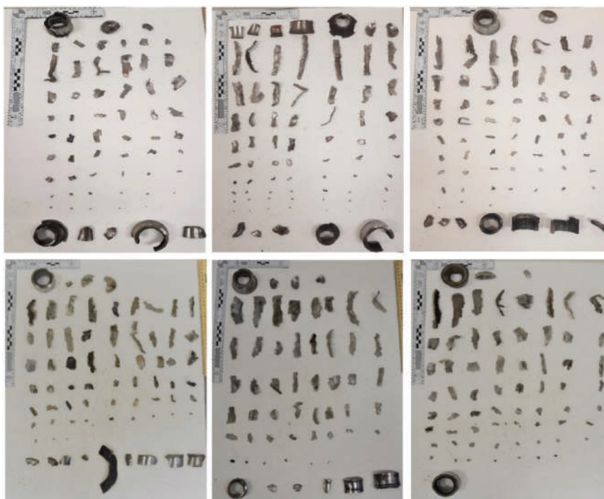
Figure 12.16 Shrapnel produced from pipe bombs. (Reproduced with permission from da Silva, L.A., S. Johnson, R. Critchley, J. Clements, K. Norris, and C. Stennett, Experimental fragmentation of pipe bombs with varying case thickness, Forensic Science International 306 (2020). Copyright Elsevier.)
