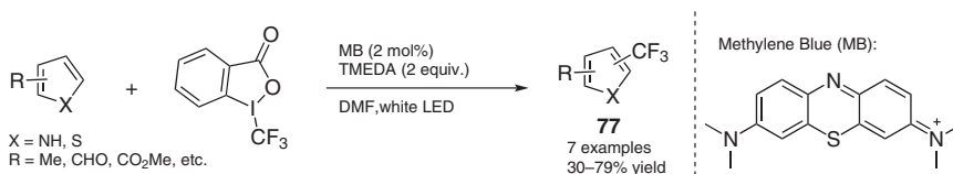
Scheme 6.30 Photocatalytic C–H trifluoromethylations. Source : Pitre et al. [72].
