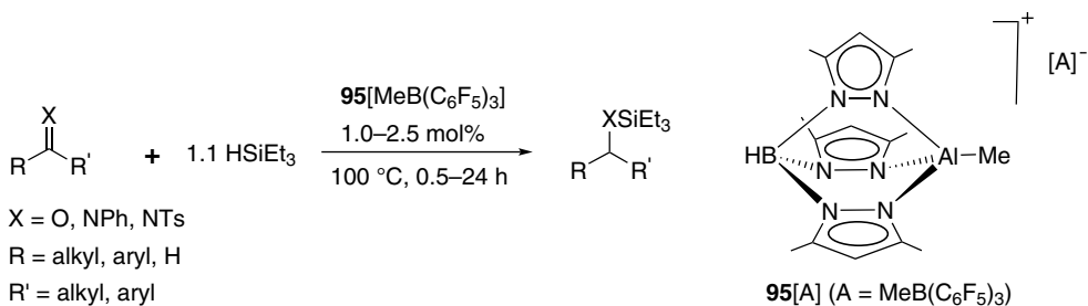
Scheme 5.39 Hydrosilylation of carbonyls and imines catalyzed by complex 95 [MeB(C 6 F 5 ) 3 ].
