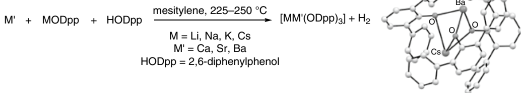
Scheme 3.19 Synthetic route to heterobimetallic diphenylphenoxides and the structure of a representative caesium bariate complex. Source: Adapted from Zuniga et al. [238].
