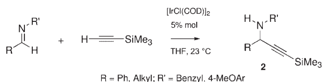
Scheme 6.1 Synthesis of a PLA by use of an Ir(I) catalyst.
