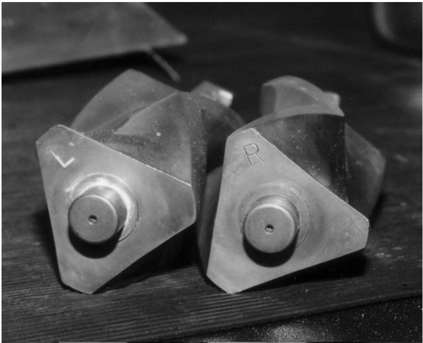
Figure 1-5 Intermeshing Rotors from Internal Mixer
