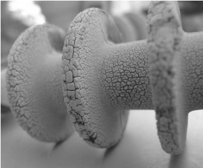
Figure 10-15 Example of Severely Degraded Elastomeric Insulator
