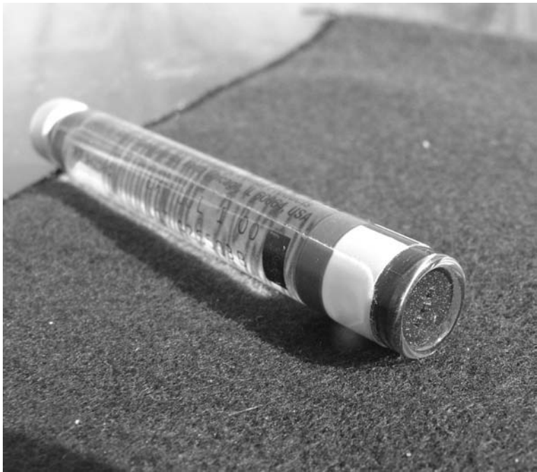
Figure 10-1 Crimped Diaphragm on Pre-Filled Syringe Vial
