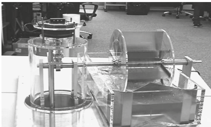
FIGURE 16.22 Water mill generator utilizing EPAM.
