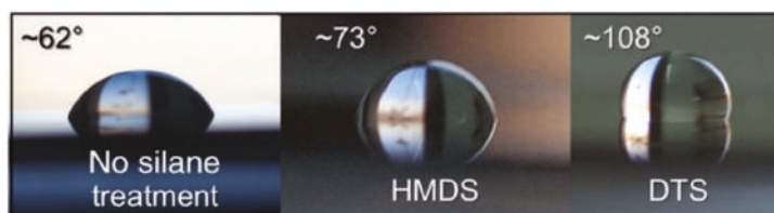
FIGURE 16.6 Water contact angles on HMDS and DTS-treated Si chip surfaces.
