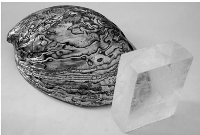
Figure 14.6. A polished abalone (paua) shell from New Zealand (left) and a crystal of the mineral calcite (right). Both materials are constructed from calcium carbonate, but in the abalone shell, the material takes the form of many layers, each a few hundred nanometers thick. These otherwise clear layers diffract light to impart the vivid colors seen in the shell.
