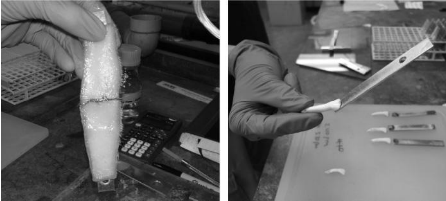
Figure 13.12. Using synthetic polymer mimics of mussel adhesives to bond together two strips of wet pig skin (left) and a cow tooth to aluminum (right). You can see the polymeric adhesive between the skin strips as well as between the tooth and metal.
