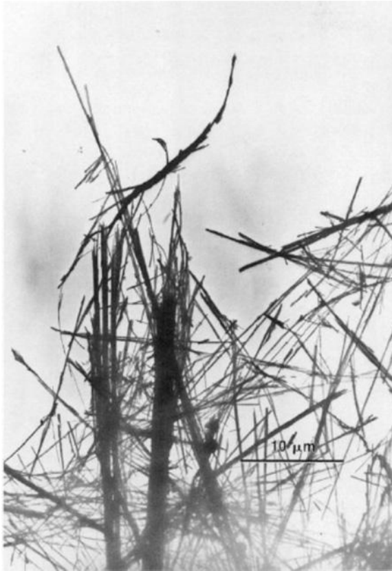
Figure 14.11. Nanofibers of the natural mineral crocidolite—one of the most toxic asbestos minerals. Source: Longo, W. E.; Rigler, M. W.; Slade, J. Cancer Research 1995, 55, 2232–2235.
