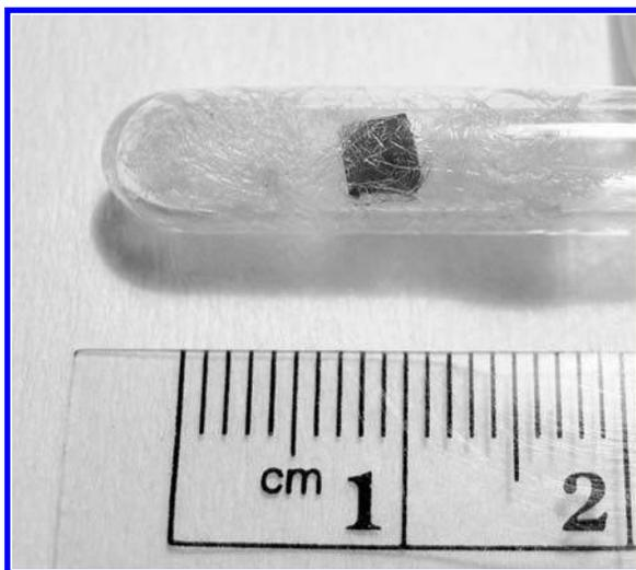
**FIGURE 3.4** Air-sensitive single crystal sample sealed in a quartz tube. Plugs of quartz wool on each side of the sample help prevent it from moving in the tube during data collection.
