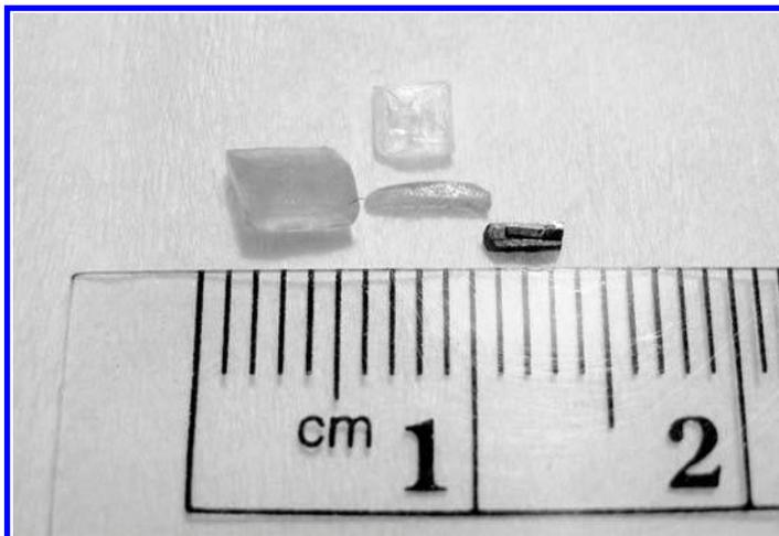
**FIGURE 3.3** (See color insert following page 86) Some representative samples from the IPNS. Although a minimum sample size of approximately  $1 \text{ mm}^3$  in volume is required for the typical single crystal experiment, in practice larger samples are often desirable.
