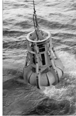
Fig. 1.7 A Russian hydraulically operated, video-directed seabed grab recovering a bottom sample from a coral carbonate mound in the Porcupine Seabight.
