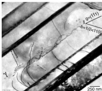
Figure 6.27 Dislocation loops in a \gamma lamella. The loops were probably left from an \alpha_2/\gamma interface that was originally present at the position of the loops. The \alpha_2 lamella was
