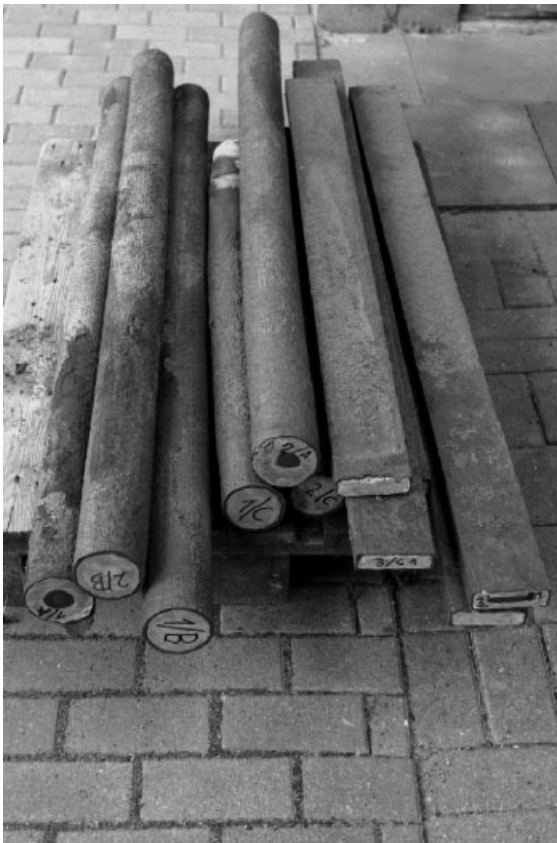
Figure 16.39 Sections of extruded Ti-45Al-(5-10)Nb-X bars that were obtained by extruding 80 kg (canned) ingots through differently shaped dies to cross-sectional reductions of 6:1 to 11:1. The extruded bars had a length of 6–8 m.
