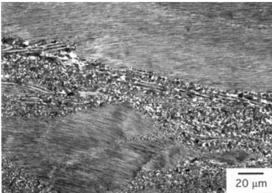
Figure 16.9 Scanning electron micrograph taken in the backscattering electron mode from a Ti-46Al alloy deformed in compression at T = 1000^\circ\text{C} and a strain rate of
