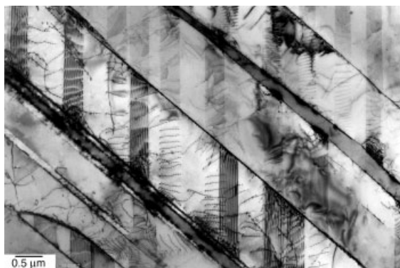
Figure 6.32 Deformation structure observed after room-temperature compression to strain \epsilon = 3.2\% showing glide of ordinary dislocations and 1/6\langle 11\bar{2} \rangle \{111\} order twinning. Ti-48Al-2Cr, as cast; fully lamellar microstructure with a preferred orientation of the lamellar interfaces parallel to the compression axis. Foil orientation axis close to \langle 101 \rangle .
