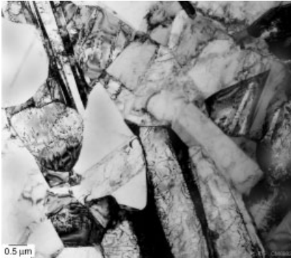
Figure 7.19 Duplex microstructure of a Ti-45Al-10Nb alloy, which had been extruded below the \alpha -transus temperature.
