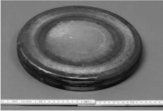
Figure 16.59 The largest TiAl disc ( \approx 32 cm in diameter and 4 cm thick) made using the novel manufacturing procedure that GKSS has developed.
