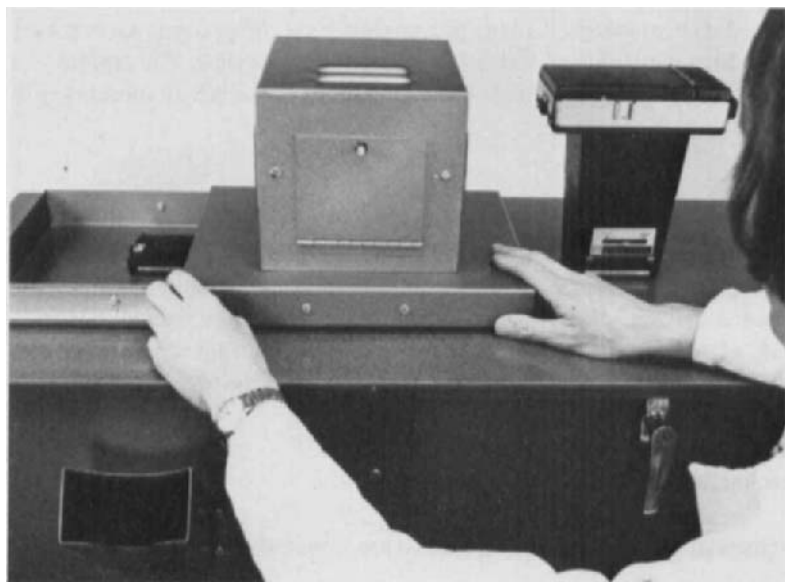
Fig. 4.21. The projector unit is removed to one side and the Polaroid camera is mounted above the projection enclosure. (Reproduced with permission from Birchover Instruments Ltd.)
