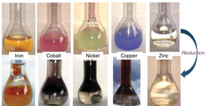
Figure 9.12 Schematic representation of metal NPs fabrication using various metallosurfactants. Source: Kaur and Mehta [30].
