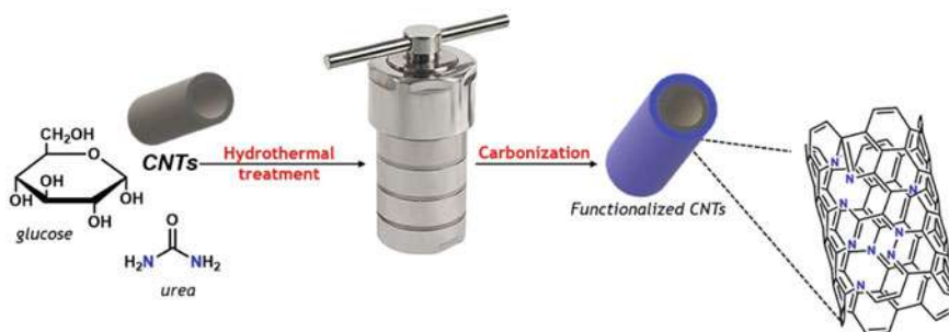
Scheme 6 Hydrothermal carbonization for nitrogen doping of CNTs
