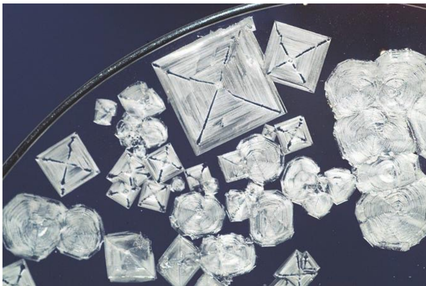
A close-up view of sodium chloride (NaCl) crystals in a water bubble within a 50-mm diameter metal loop photographed by a crew member doing research in the Destiny laboratory on the International Space Station on March 13, 2003 (NASA)
