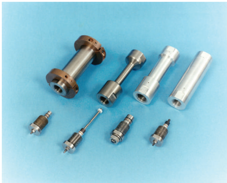
Figure 3: Selection of high pressure cells with unsupported area seals. (Credit: STFC)
