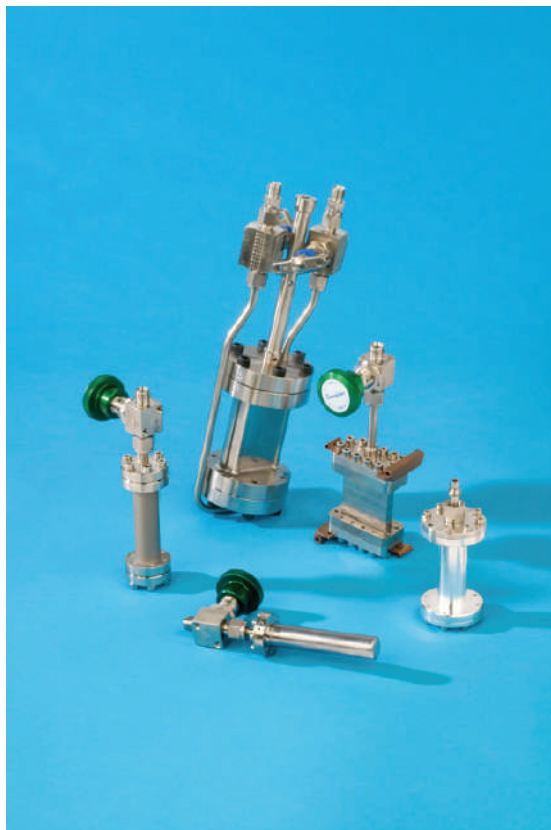
Figure 2: Selection of gas handling cells suitable for catalysis in flat plate and circular/annular geometry. To provide a sense of scale, the gas tubing on all cells is \frac{1}{4} " O.D. (Credit: STFC)
