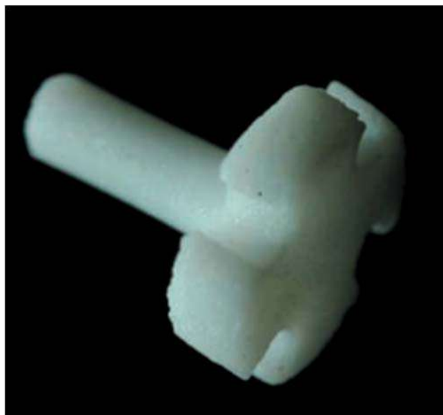
Figure 19.3 TORP made of Bioverit II. Source: Turck et al. [49], Figure 01, (p. 03)/reproduced with permission from 2007 Taylor & Francis.
