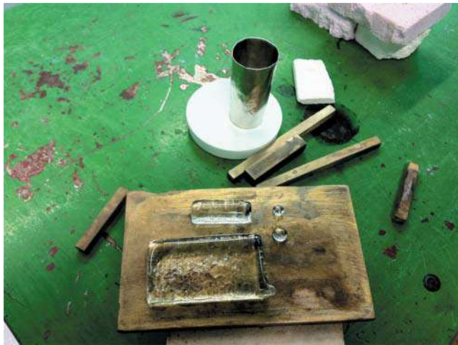
Figure 15.1 Image of a Europium-doped \text{CaSiO}_3\text{--Ca}_3(\text{PO}_4)_2 bioactive eutectic glass manufactured by the casting technique.
