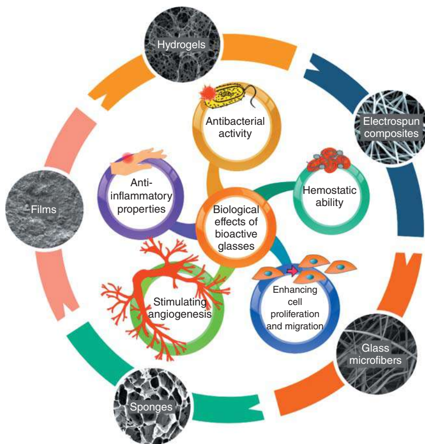
Figure 21.2 The possible biological mechanisms of bioactive glasses in wound healing and different approaches of incorporating bioactive glasses in the polymeric matrix to be used in wound treatment. Source: Tina Mehrabi (author).
