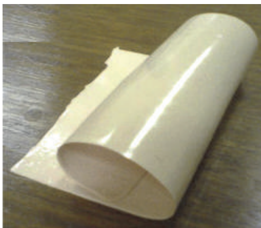
Figure 5.13. Photograph of a green GDC tape fabricated from the SCS powder. Adapted from Akbari-Fakhrabadi et al. (2012).
