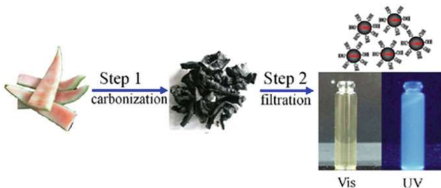
Fig. 7 Graphical abstract of water-soluble fluorescent carbon dots synthesis based on watermelon peel (By Zhou et al. [96], License number 4960330931030 provided by Elsevier and Copyright Clearance Center)
