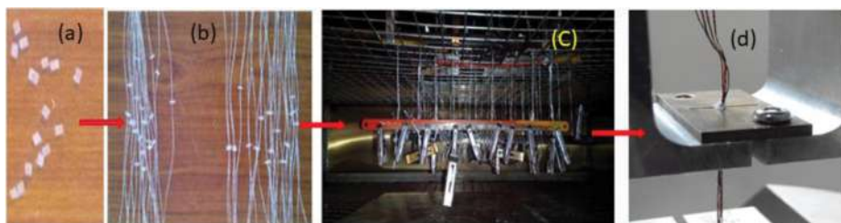
Figure 7.4: Fabrication steps: (a) matrix pieces, (b) matrix–fibre bundle assembly, (c) thermal processing, and (d) final sample gets sheared off from the bundle on microvise.
