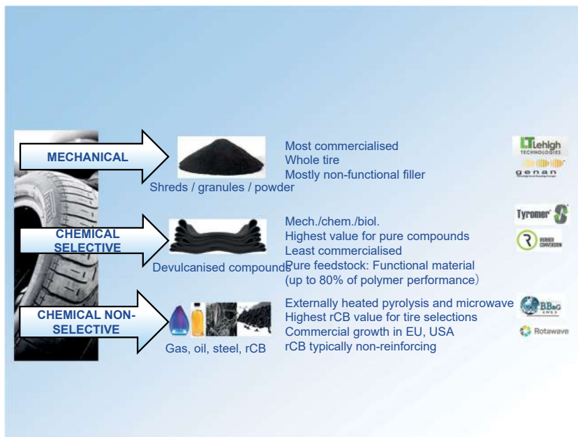
Figure 9.3: Tire recycling processes.
