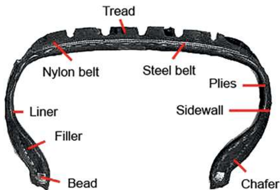
Figure 9.1: Tire cross-section.
