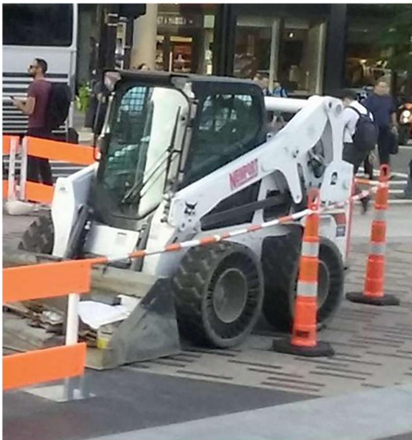
Figure 9.5: Alternative Wheels – Michelin’s Tweel®.
