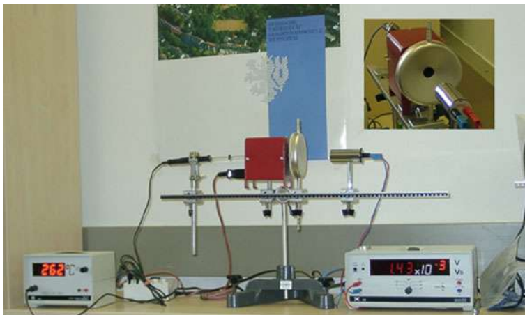
Fig. 2.3 Experimental setup in the author's office allowing to verify Stefan's law
