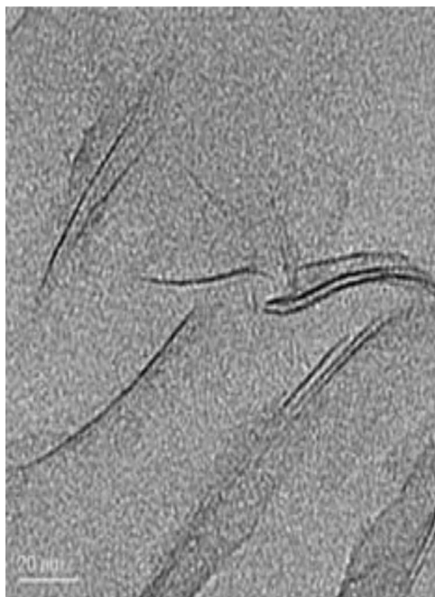
FIGURE 10.8 TEM of MMT/PMMA composite (Adapted from Prado and Bartoli 2018.)
