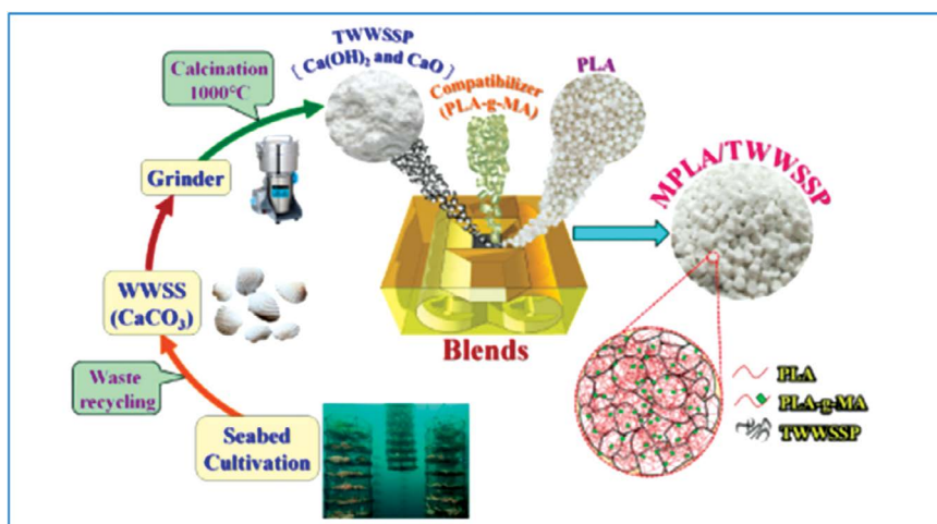
FIGURE 1.9 Preparation of PLA composites with calcined WWSP (Adapted from Wu et al., 2019.)
