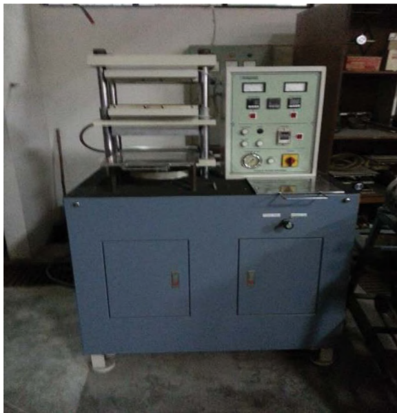
FIGURE 5.1 Compression molding machine.
